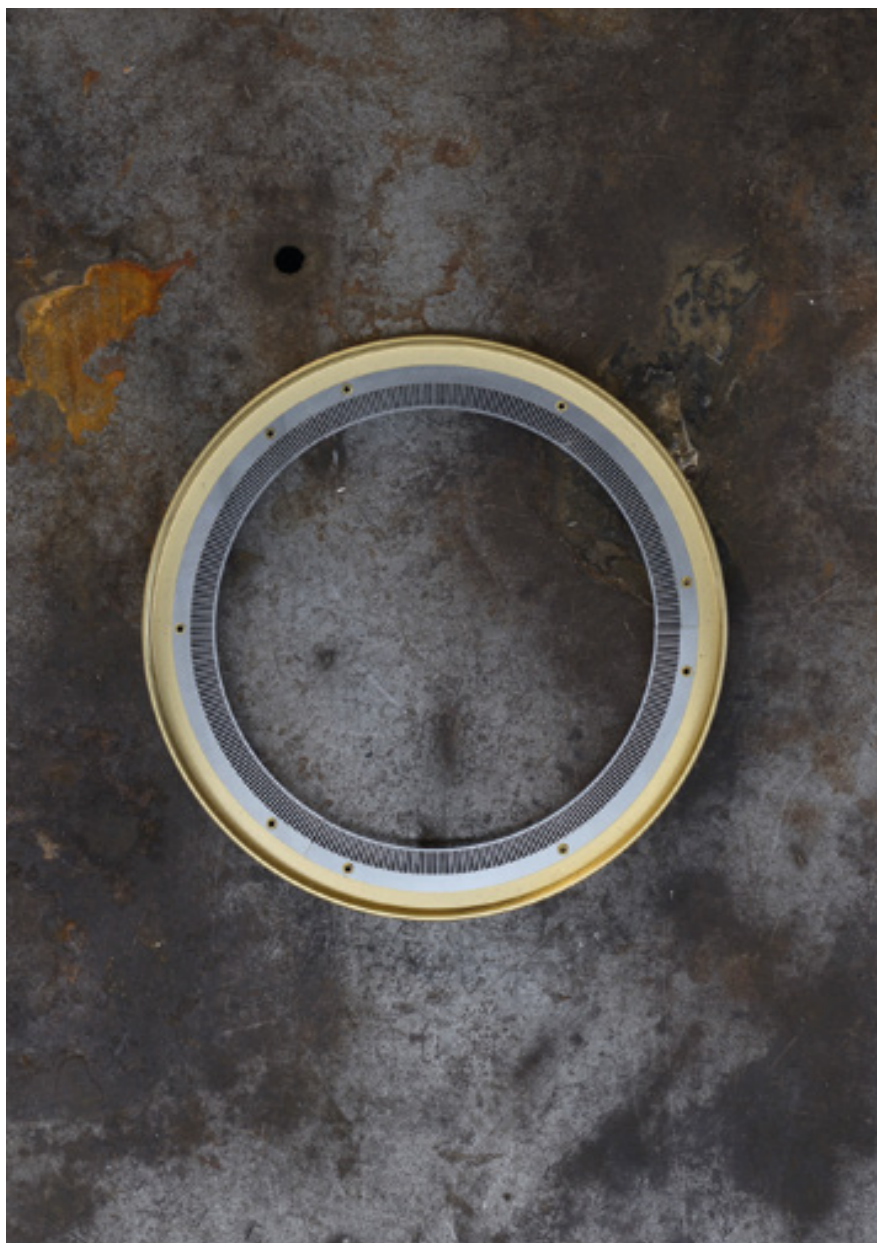
Eva's CNC turned ring with photoengraved optical wheel.
