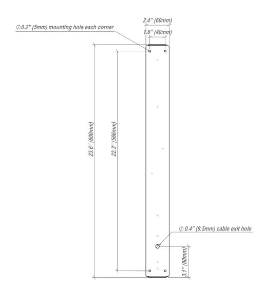
Backplates can be rotated 180 degrees- to allow cable exit to be positioned at top if required.
