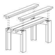
Finally, install the outer T-profiles and fix with screws and washers.
