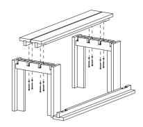
Install the central T-profiles first and fix each with four screws and washers.
